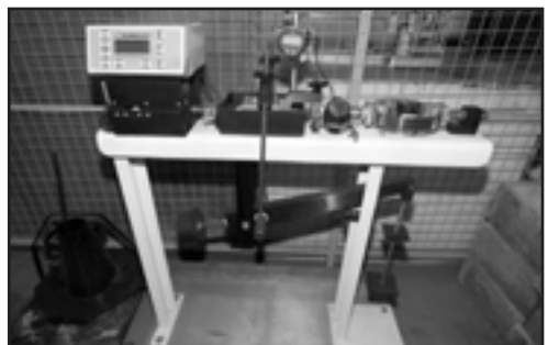
Facility for testing soil residual shear in digital format.
